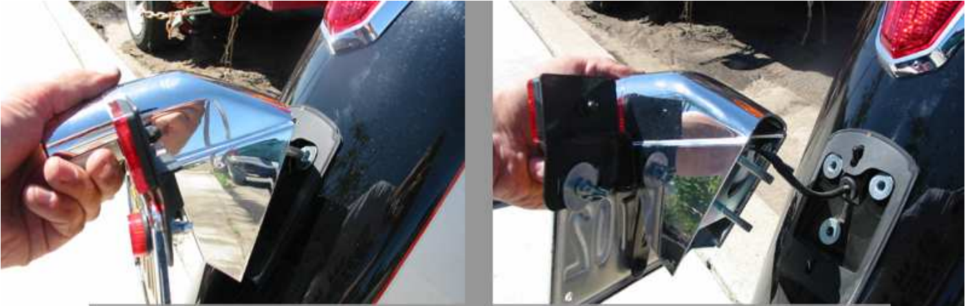
Slowly remove plate holder from rear fender. Wires will be attached.
