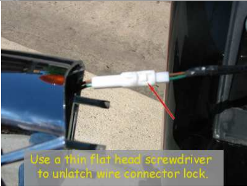
Slowly remove plate holder from rear fender. Wires will be attached.
