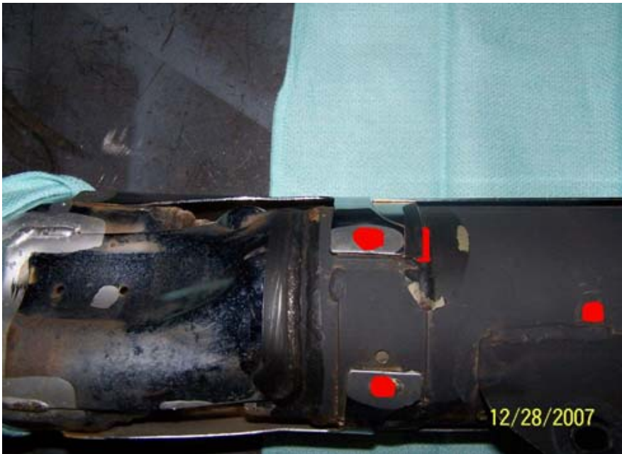
Spot welds that need to be drilled & cut with cut off wheel
