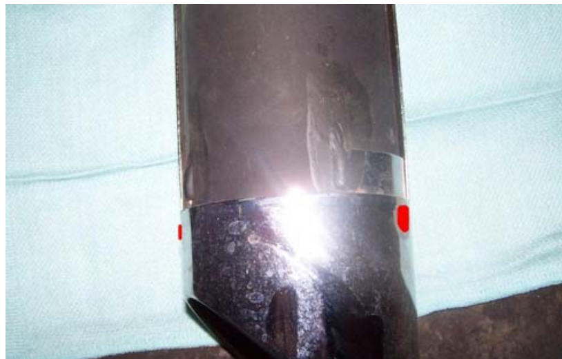
Drill the 2 spot welds, one on top and one on bottom to remove the rear cover
