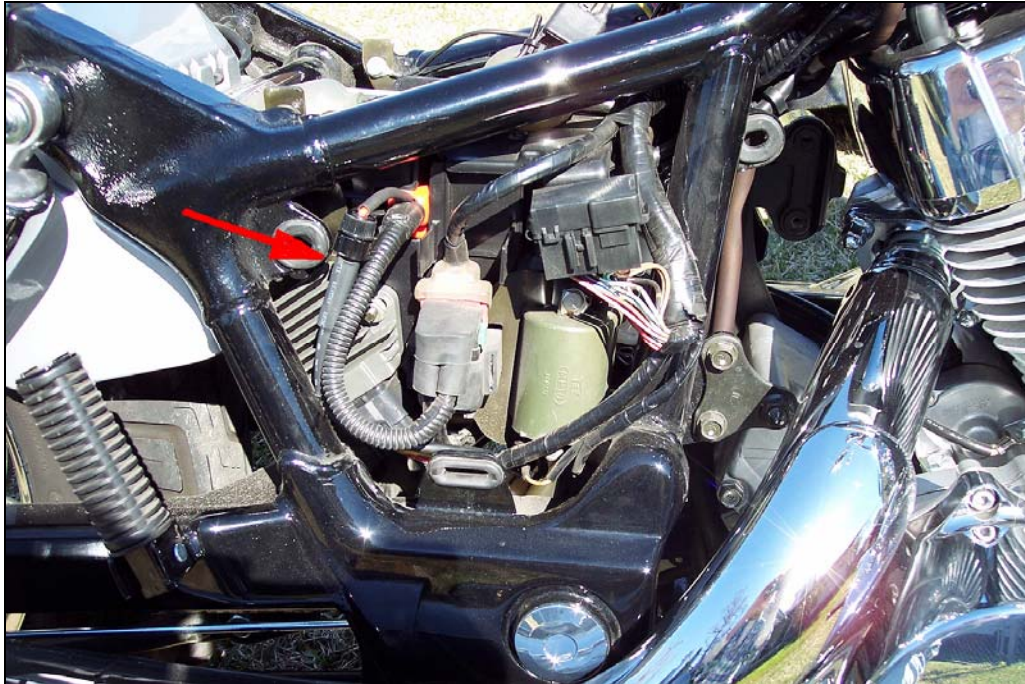
In-Line Fuse From Battery to Relay
